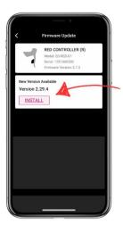
7) Press and release the component's AXS button to begin the firmware update. The component's orange/amber LED will flash rapidly, and the app will display the update progress.
